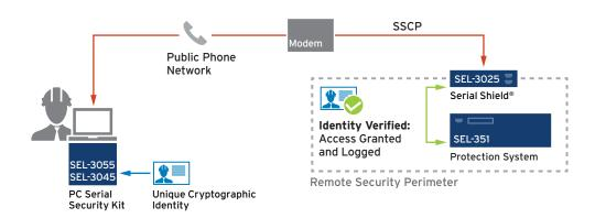
Secure machine-to-machine connections with SEP, and easily manage remote SEL-3025 Serial Shields over Ethernet or serial links. SEP supports a variety of bit- and byte-based protocols, including DNP3, Modbus® RTU, IEC 60870, Conitel, and more.
