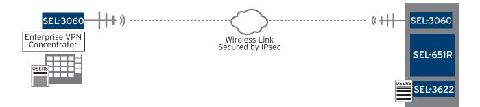
Secure all Ethernet and serial data communications with IPsec or SSH.
