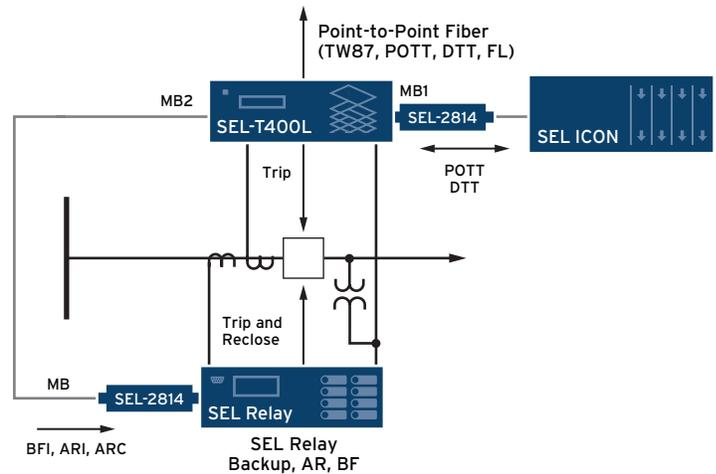
This is a recommended all-SEL application of the SEL-T400L. Use the SEL-421 Protection, Automation, and Control System or SEL-411L Advanced Line Differential Protection, Automation, and Control System for backup protection, breaker failure protection, and autoreclose functions.
