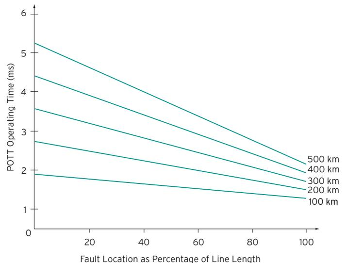
POTT operating time as a function of fault location, as a percentage of line length, assuming a point-to-point fiber-optic channel.
