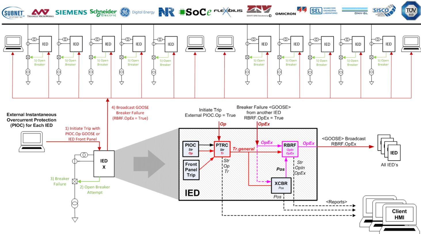
IEC 61850 Breaker Failure Demonstration – Application Diagram
