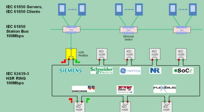
IEC 62439-3 HSR Network Redundancy Interoperability Demonstration at UCAIUG Booth
