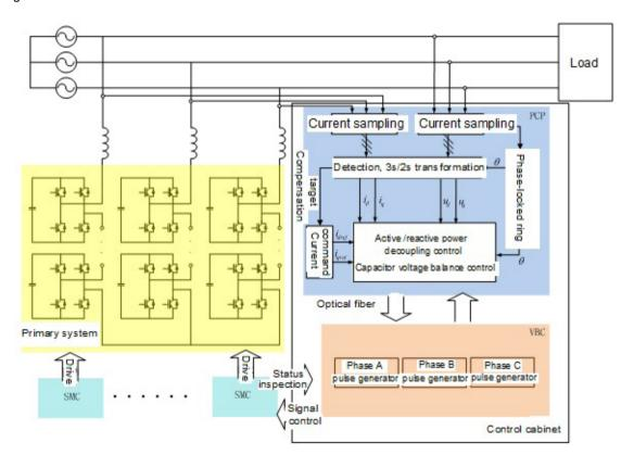
The upper control uses the common decoupling control algorithm:let the d-axis responsible for the active power to achieve the stable control of the DC side capacitor;letthe q-axis responsible for the reactive power to achieve the control of the reactive power need of the system. To realize the DC capacitor balance algorithmof the chain link, the balance control algorithm can be added on the basis of modulation wave to ensure the balance of the DC side capacitor voltage.
