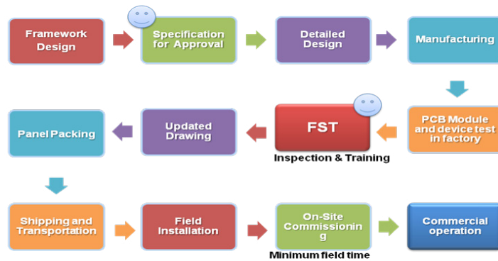
Figure 14 work flow and Quality assurance
