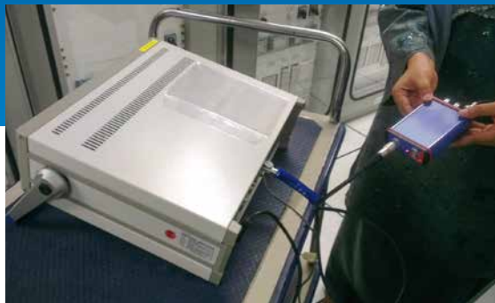
Time synchronization with CMIRIG-B: CMC 256plus is synchronized with the time server along with the devices under test.
