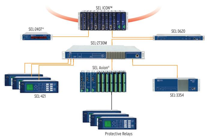
In this example of a substation network, the SEL-2730M supports engineering access from the SEL-3354 Embedded Automation Computing Platform and aggregates IEC 61850 traffic from the SEL-2240 Axion® and SEL-421 Protection, Automation, and Control Systems.
