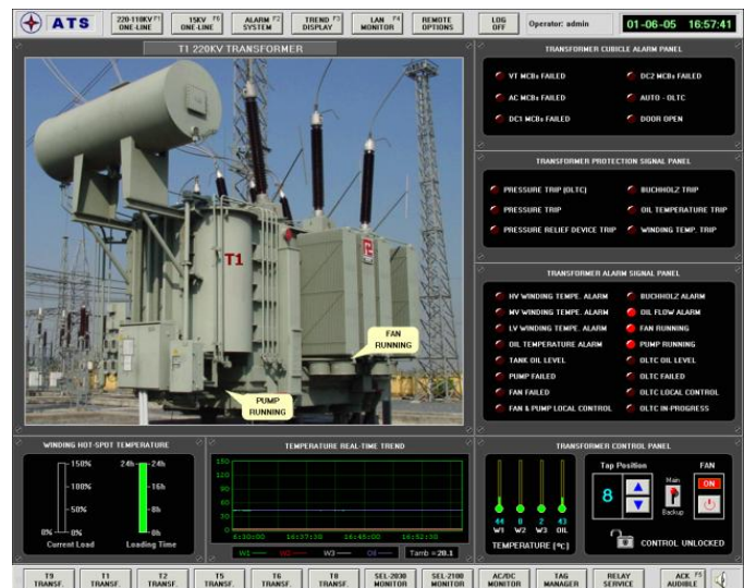
Fig. 10. Detailed Display of 220 kV Transformer
