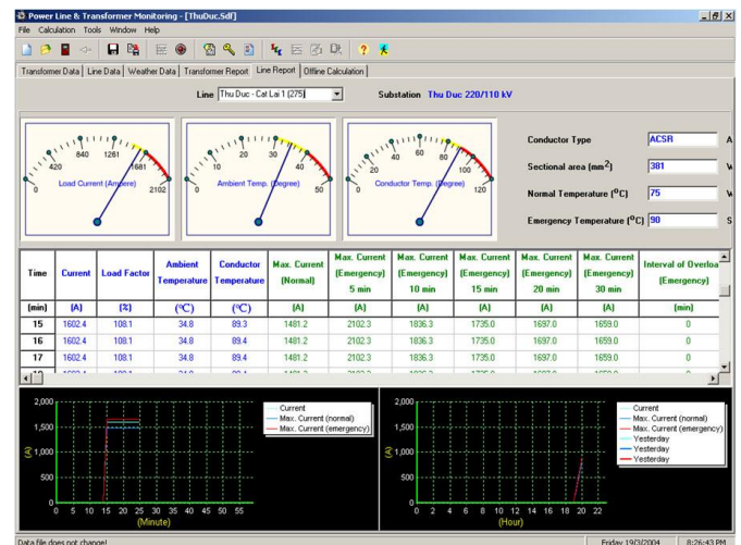
Fig. 12. Dynamic Loading Capacity User Interface
