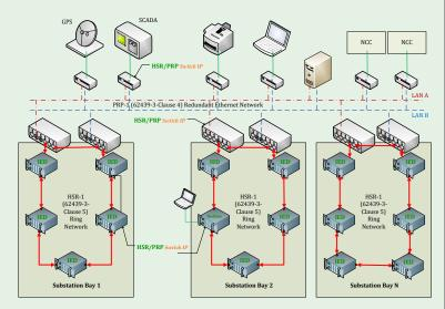
The two Ethernet networks (LAN A and LAN B) are independent. DAN nodes connect to both LANs and send the same frames over both networks. Destination nodes consume the first received frame and discard the duplicates.
