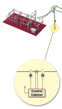
In order to improve the operational efficiency and reliability of the overhead MV distribution grids, utility companies need to consider automation solutions for the switch disconnectors as well as circuit breakers. These type of solutions allow to divide MV lines into several sections, and provide the capability to insulate the faults automatically or via remote control.
