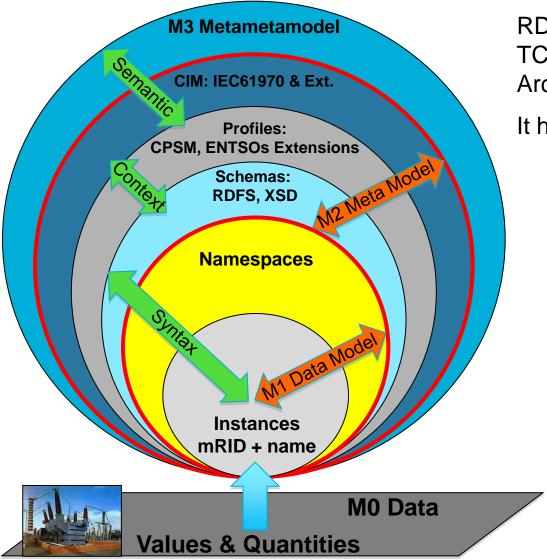
RDF/XML layers combined with TC57 Layered Reference Architecture
